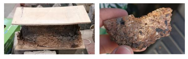
Figure 11 - Photos of bricks after crushing. New brick (L), Reclaimed brick (R)
