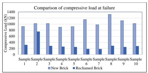
Figure 8 - Column chart displaying load at failure for both sample sets.
