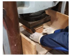
*Figure 3 - Image of prepared new sample being placed into testing machine*
