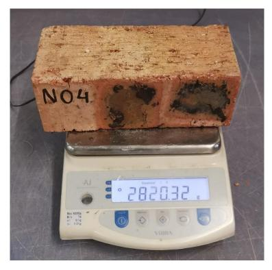
Appendix Y - AJ-6200E precision balance machine used to weight the samples
