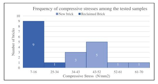
*Figure 10 - Histogram showing spread of compressive stresses among the samples.*
