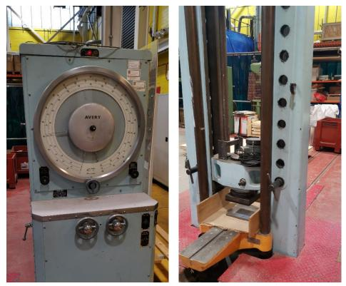
Figure 4 - Avery analogue compressive testing machine used for the reclaimed bricks
